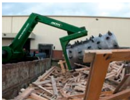
Mammoth Roll Packers Ideal for compacting large, bulky and medium density materials.
