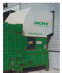
Through wall chute fed
